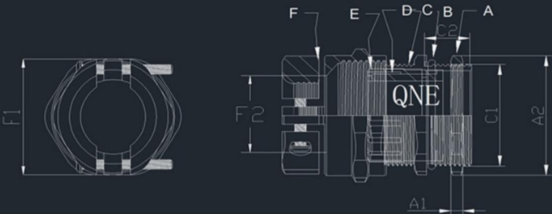
**Thread:** Metric, PG, G(PF/BSP/PS), and NPT thread
